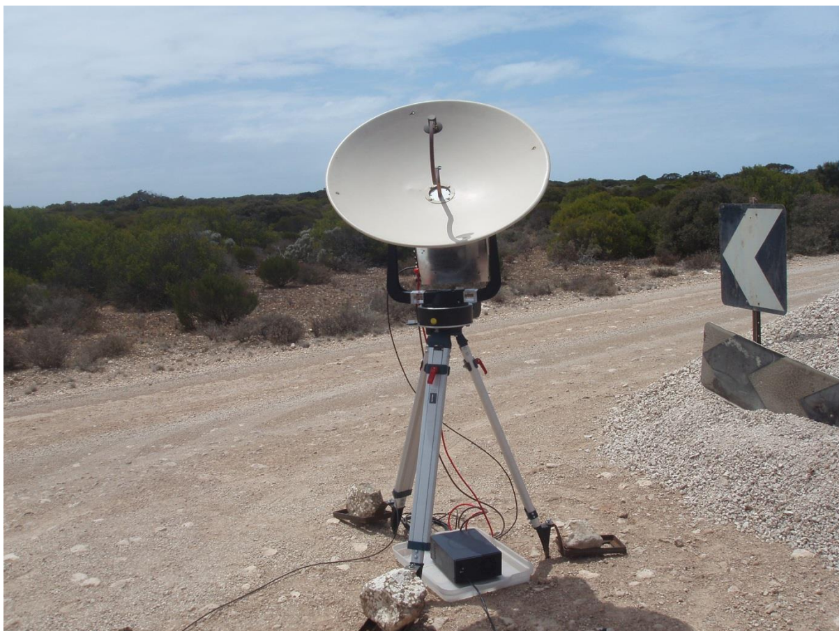
Fig. 2 — The VK7MO portable setup for 10 GHz EME.
