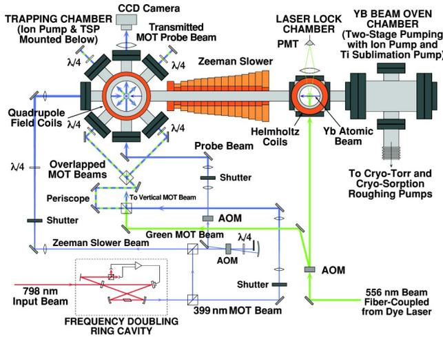
FIG. 2. Diagram of the Yb MOT apparatus.
